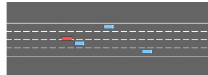
Fig. 8. HighwayEnv: a transition is labeled unsafe when the ego vehicle comes within distance 0.2 of another vehicle.
