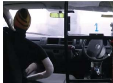
Figure 38 Minibus steering control system with a dummy being tested.
