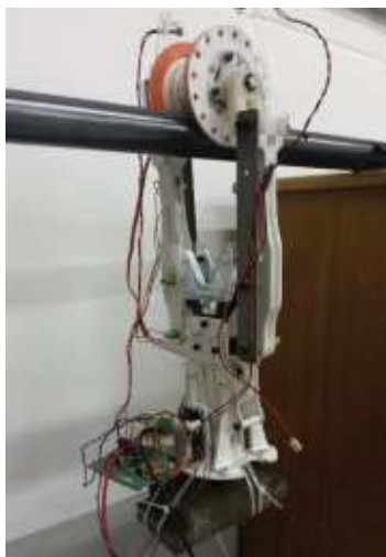
Figure 35 Brachiating robot gripper/pulley.
