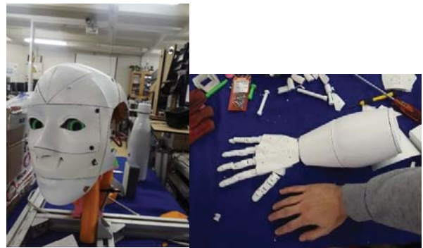
Figure 3 A 3D printed fully functional head, arm and hand developed as part of the humanoid robot project.
