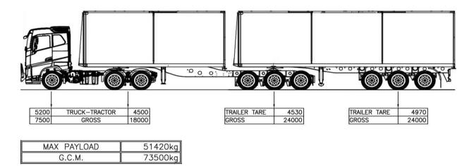
Figure 1: Typical PBS B-Double configuration
